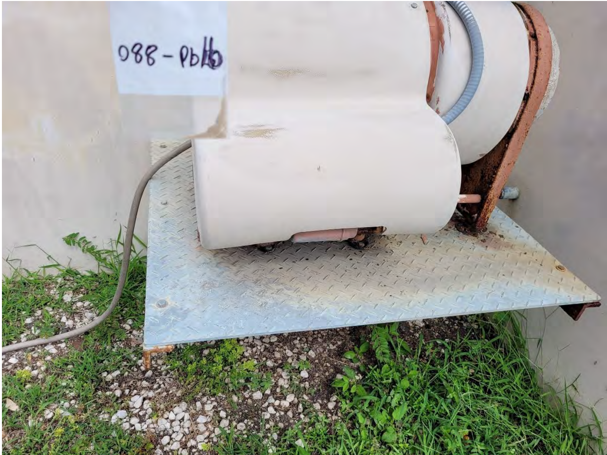
088-PB 16: Beige Paint on Fiberglass Motor Cover [NLD]
