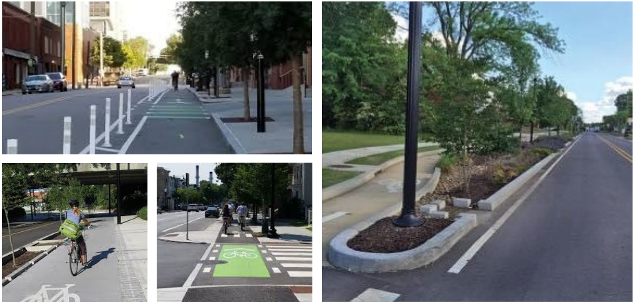
Figure 6: Examples of Separated Bike Lanes, including crossing markings and LID Measures
